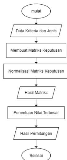
Gambar 1. FlowChart Metode Simple Additive Weighting
